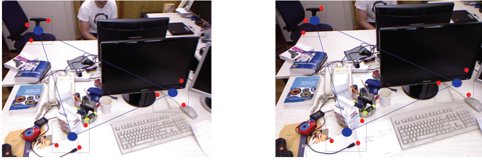
Fig. 5 Pixel positions of 3 scene sections with their centers. The center pixel positions are calculated by averaging the pixel positions of the matched features within each section.
