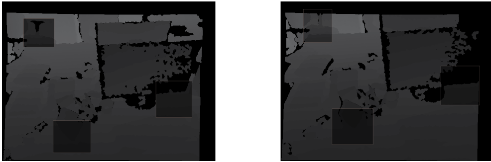
Fig. 6 Depth is calculated from neighbour image patches. Note that not the entire section is used to calculate depth, only the neighbourhood of the matched features within the section.
