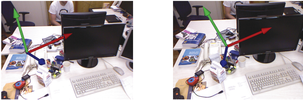
Fig. 8 Scene models in the previous and latest frames. As the camera moves, it views the scene from a different pose therefore the scene appears to move relative to the camera. The scene model follows this relative motion.
